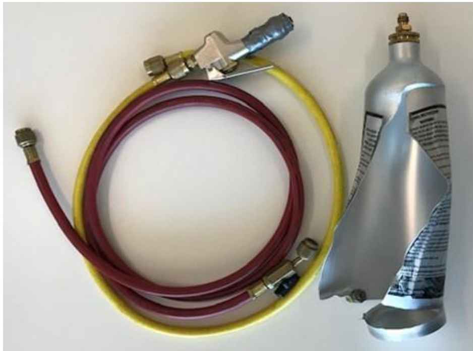
Example of a ruptured flushing canister. Provided by NT WorkSafe.
