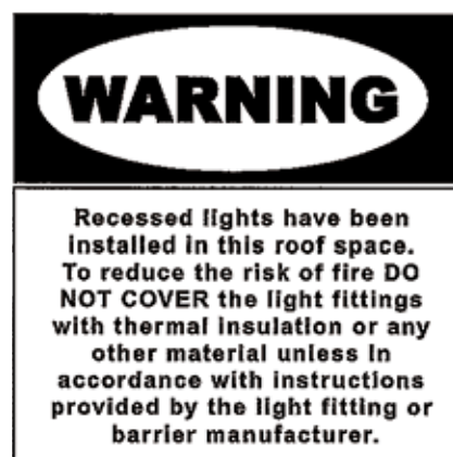
Figure 4.8 Warning sign to be installed in accessible roof spaces containing recessed luminaires
