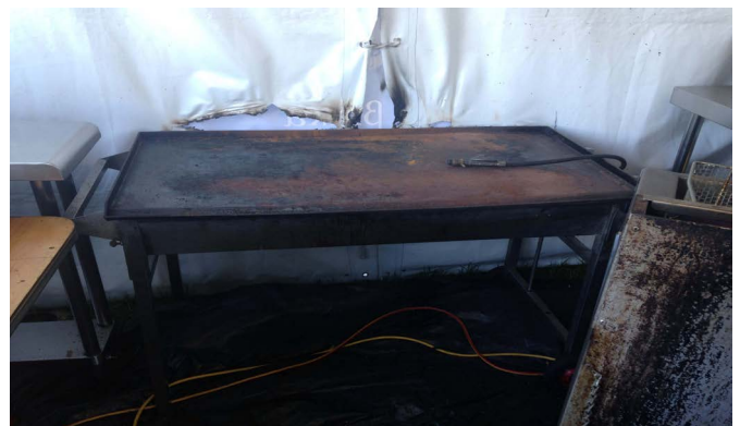
Plastic marquee damaged after touching gas fired solid grill plate
