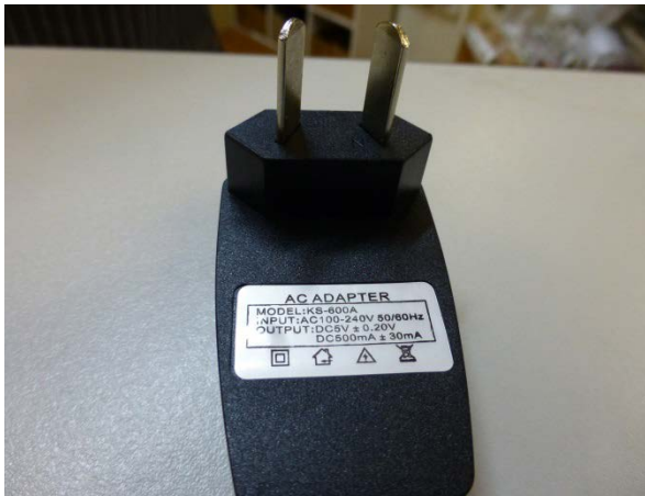
Unapproved USB adapter (note the uninsulated pins)
