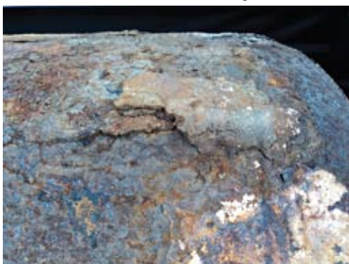
Showing the LP Gas fuel container with heavy corrosion
