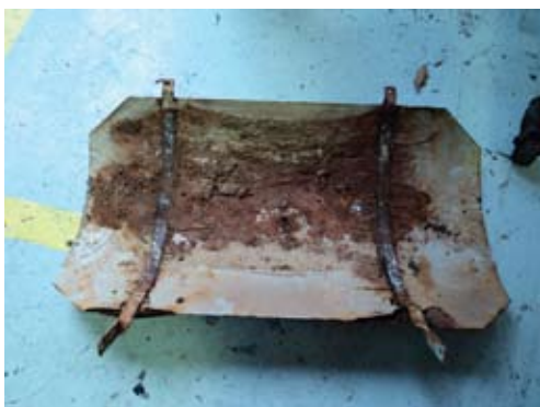
Showing inside of the container guard. Note the sand and other foreign material.
