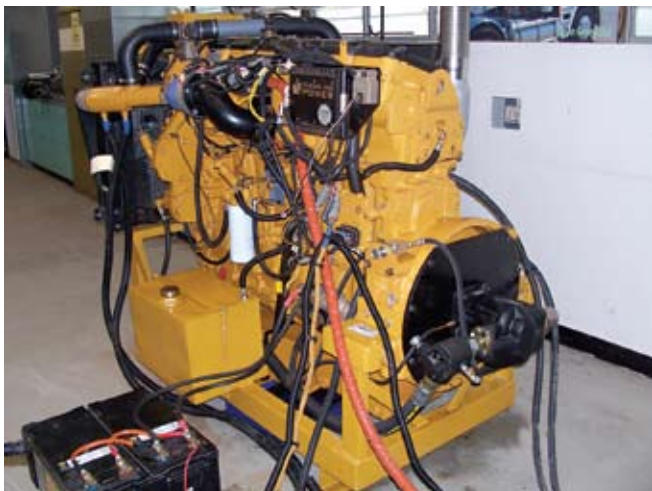
15 Litre Caterpillar (C15) engine converted to LNG as used in road transport vehicles (Flat Liner)
