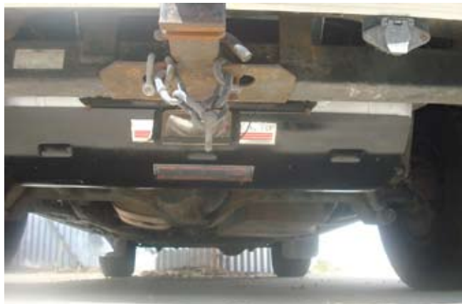
Showing underslung LP Gas fuel container and guard
