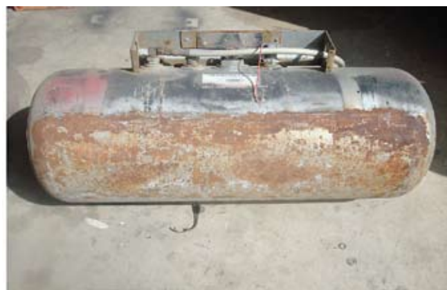
Showing heavy corrosion under guard
