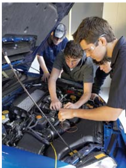
Trainees working on an Auto LP Gas system. (Photo courtesy of Challenger Institute)
